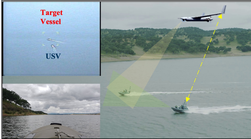
Clockwise from bottom left: Mokai USV FPV image; ScanEagle aerial image of USV pursuing target vessel; SeaFox USVs on Lake San Antonio
