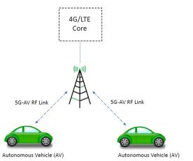
Block diagram that shows the communications between autonomous vehicles to a 5G tower. The 5G tower is anchored to the 4G/LTE core, as defined in the 5G NSA architecture
