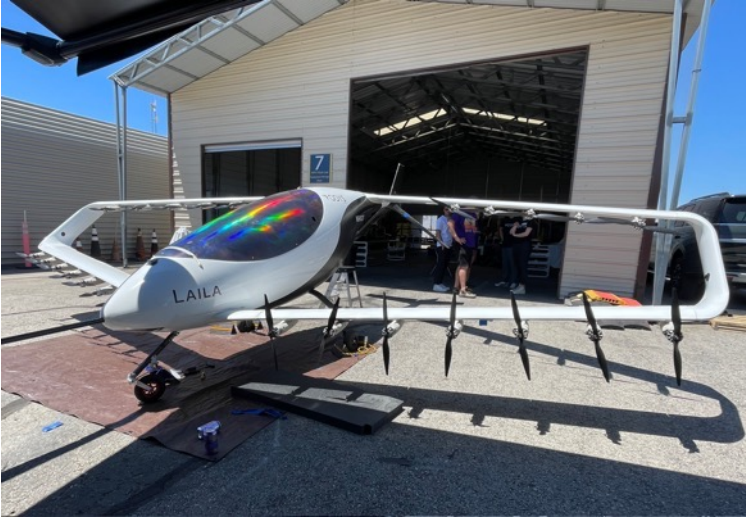
Odys Aviation validated the ability to transport and rapidly prepare, Laila, their twenty-one-foot box wing VTOL prototype aircraft from container to fully assembled in less than thirty minutes.
