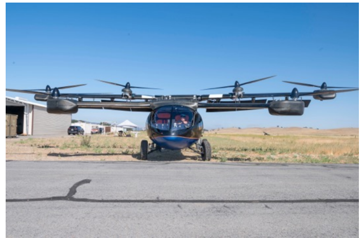
The ASKA team demonstrates how the wings open and close on their prototype A5, flying car. With wings folded the A5 is street legal.
