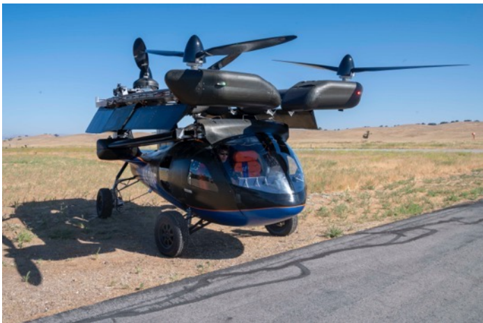
The ASKA team demonstrates how the wings open and close on their prototype A5, flying car. With wings folded the A5 is street legal.
