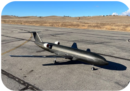
A-04: M4 Engineering, Inc experimented on their all-electric subscale remotely-piloted flight test vehicle.
