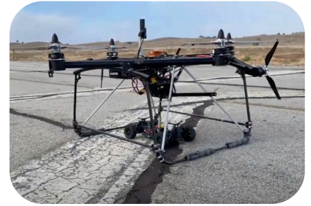
A-05: Toofon tested payload delivery by carrying a small UGV on their long-range, heavy-lift vehicle.
