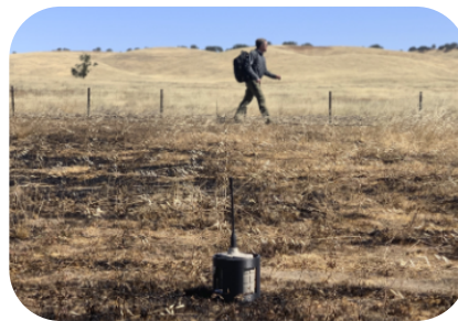
F-02: Innovative Algorithm's Seismic Sensor identifies a person of interest crossing the border
