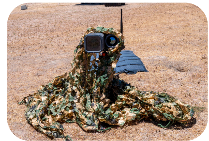
D-03: Gantz-Mountain conducted automated object detection and classification using both long-range and thermal cameras
