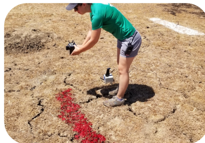
A-02: Spectrabotics used their hyperspectral sensor to classify the powdered material that was dropped by the person of interest
