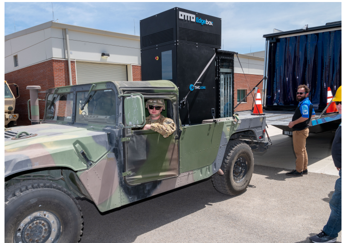
J-01: TMGCore tested their portable data center's ruggedness by placing it on a HMMWV at Camp Roberts.
