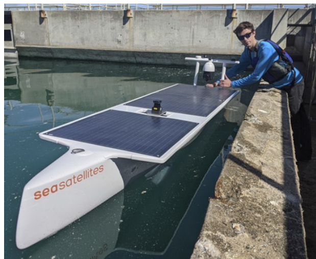
F-04: SeaSats deploy their unmanned surface vehicle with persistent ISR capabilities to detect a vessel of interest.
