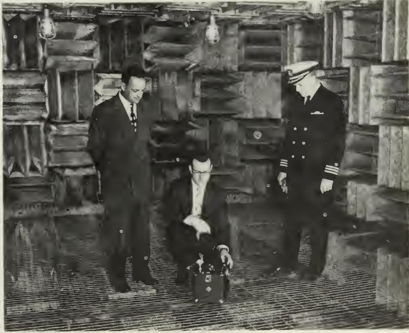
Taking measurements of sound in the Anechoic Chamber.
