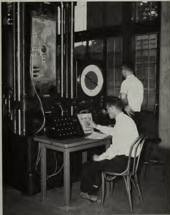
Conducting tension tests at the Naval Postgraduate School's mechanical engineering laboratory are LT Donald B. Davis (seated) and LT Lawrence J. Opezio, both of the Coast Guard. An important part of the mission of the School is to foster research as a means of offering stimulating educational opportunities to students.
