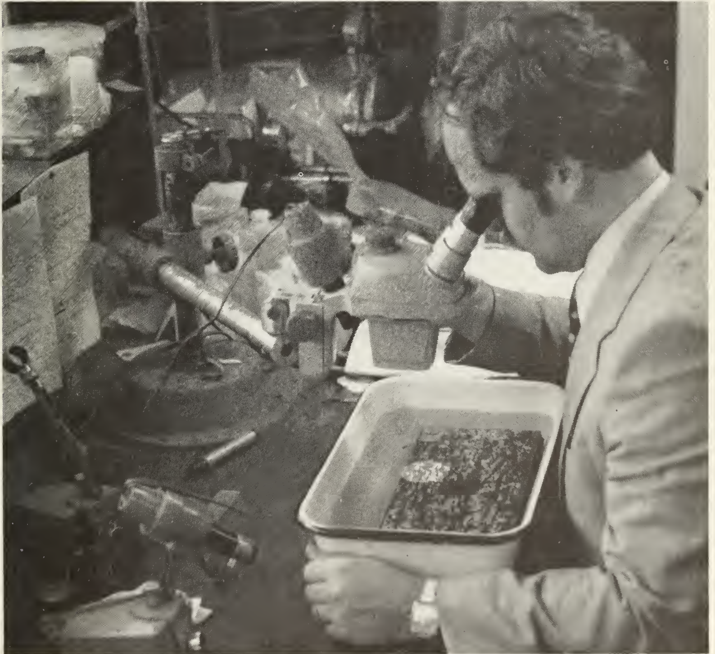
Student examining typical fouling organisms on experimental surfaces
