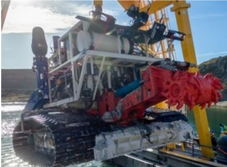
Figure 17. Seabed crawler as tested by the iVAMOS! Consortium, October 2017. 17
